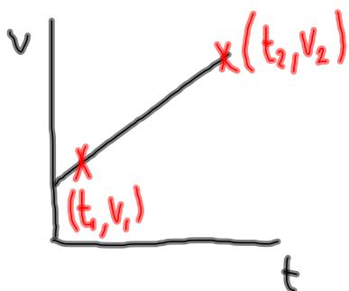
$$\text{slope} = \frac{\Delta v}{\Delta t} \quad \begin{matrix} \text{rise} \\ \text{run} \end{matrix}$$
